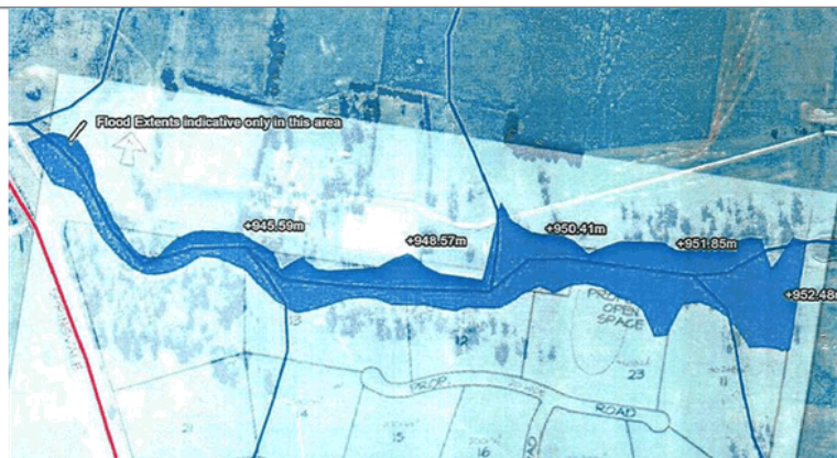
Figure.6 Flood affected lands, northern watercourse
